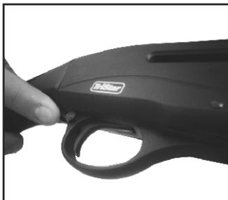
**C.** When you are ready to fire the gun, press the safety button to the "off" or "fire" position, so that the safety protrudes from the left side of the gun and the **RED BAND MARKING IS SHOWING**.
