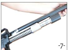
7. Remove the barrel to the rear slightly
