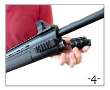
4. Unscrew the front handguard secure cap and remove it
