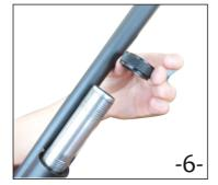
6. After you remove the Forearm, push "Cartridge Ramp Lock Button" and remove "Fixing Nut Barrel"
